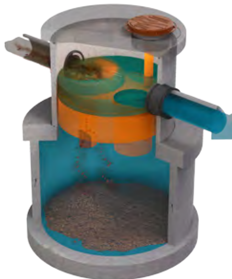
Figure 2 – HumeCeptor® system operation during high flow conditions
